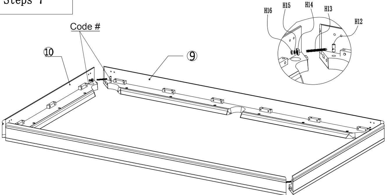
**Attention:** There are some code number(#--#) writing on both bottom ends of each short and long rails, please connect 2 rail ends together correspondingly with the same code # by sequence in order to avoid some big gap between each 2 ends.
