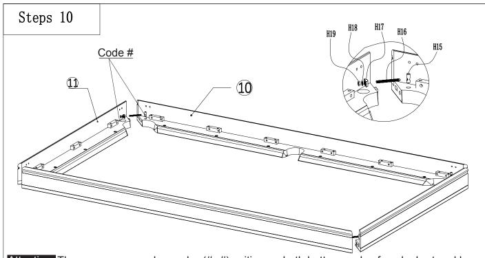
Attention: There are some code number(#--#) writing on both bottom ends of each short and long rails, please connect 2 rail ends together correspondingly with the same code # by sequence in order to avoid some big gap between each 2 ends.
