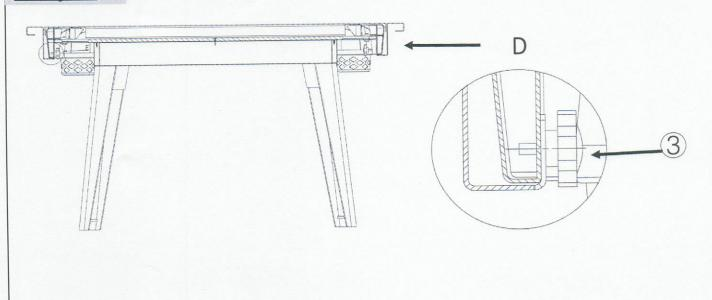
Place the Clamp (D) with the Table (A) and Table Top (C), using Screws (3).
