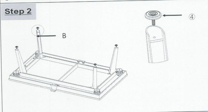
Place the Adjustable foot levelers (4) with the Table Legs (B). Note: If the floor is not flat, the table will be easily shacking after installation or the balls could not roll properly. If in this case, please adjust the foot levelers (4) until the playfield is in level status.
