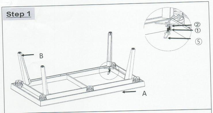
Place the Table upside down (A) onto a clean, non-marring surface. (Note: Be careful as any sharp and hard object may damage the surface of the product.) . Attach the Table Legs (B) the Table Reverse Side (A) as pictured, using Screws (1), Washer (2) and Spanner (5) until they are very tight together.
