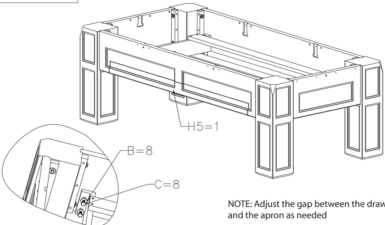
NOTE: Adjust the gap between the drawer and the apron as needed
