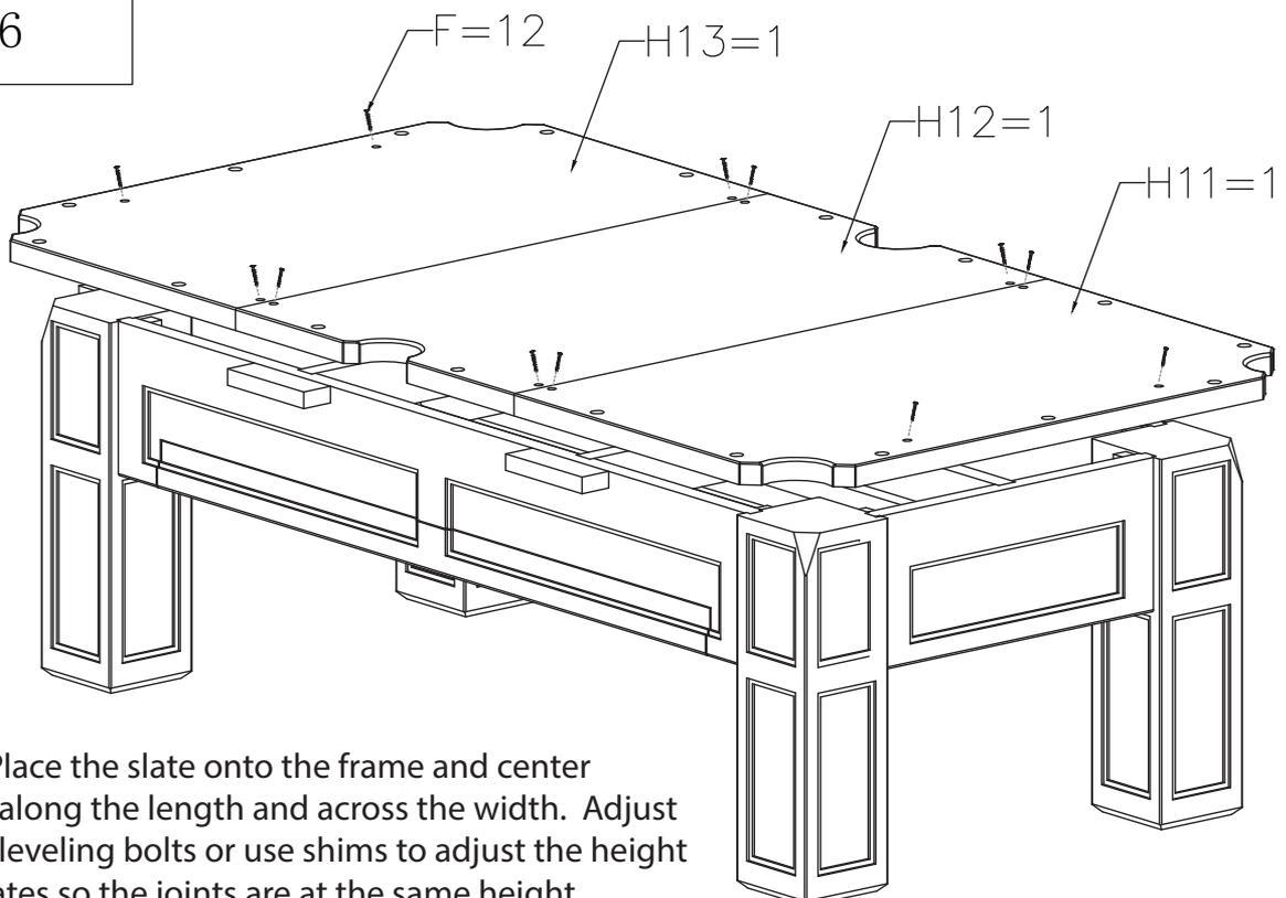
NOTE: Place the slate onto the frame and center carefully along the length and across the width. Adjust the slate leveling bolts or use shims to adjust the height of the slates so the joints are at the same height
