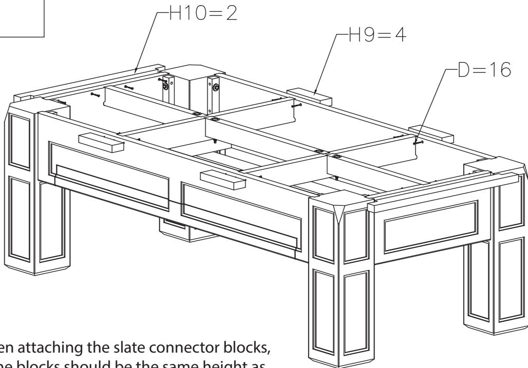
NOTE: When attaching the slate connector blocks, the top of the blocks should be the same height as the top of the apron. They should not be higher than the apron
