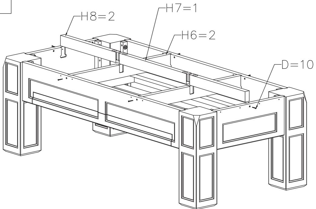
NOTE: The tops of the cross beam supports must be at the same height as the tops of the aprons and legs
