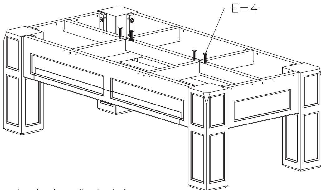
NOTE: When inserting the slate adjusting bolts, the head of the bolt should be even with the top of the cross support or slightly below. It should not be higher than the top of the cross support
