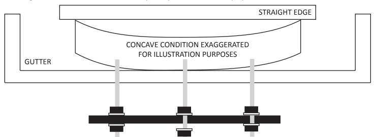
Once the desired adjustment has been made continue to the next climatic adjuster and repeat the process
