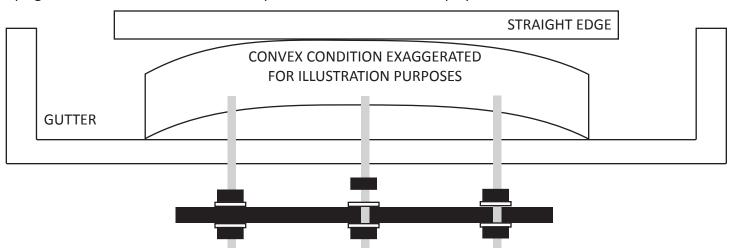
To correct a concave playfield loosen the nut below the metal bar. Slowly tighten the nut above the metal bar down against the washer and metal bar to push up the center of the playfield.
