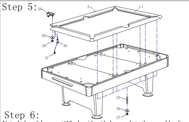
Note: It doesn't have part#19 when it's with drop pockets, the assembly of part#19 is only available for the table with ball return system. Install part#19 and part#24 when it's with ball return system. But install part#48 instead of part#24 and install part#46 when it's with drop pockets.
